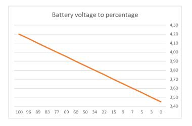
As a rule-of-thumb, Li-Po batteries are complex thus the exact charge may differ slightly depending on varying factors like load, temperature, humidity etc.
