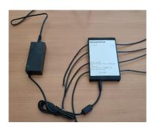
Take the plug of the battery that needs to be charged and the StreamLine Spider charging port (5). Orient the plug and the port so that the pieces that stick out line up as in the picture below. Connect the battery to the charging port.
